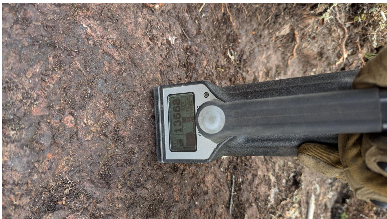
Figure 4. Newly discovered hematized magnetite-rich pegmatitic orthogneiss reaching upwards of 13,500 cps, in the T-Lake area.
