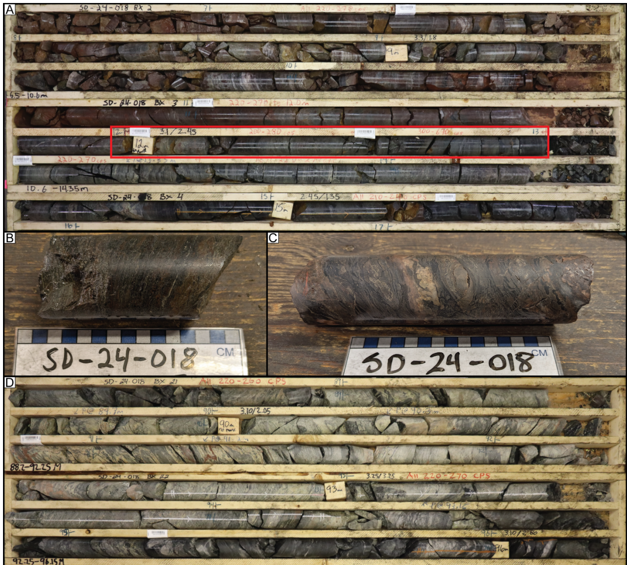
Figure 4. Drill core photos from hole SD-24-018 highlighting intervals of anomalous radioactivity, alteration and structure. A) Faulted and hematite-limonite-altered hangingwall rocks hosting radioactivity up to 1,582 cps at 12.5 m. B) Close-up of sheared and altered semipelitic gneiss hosting radioactivity up to 1,582 cps. C) Close-up of deformed pelitic rock hosting radioactivity up to 835 cps at 22.7 m. D) Strong sericite-clay and hematite alteration overprinting a graphitic shear zone; Up to 270 cps, from 88.2 to 96.15 m.
