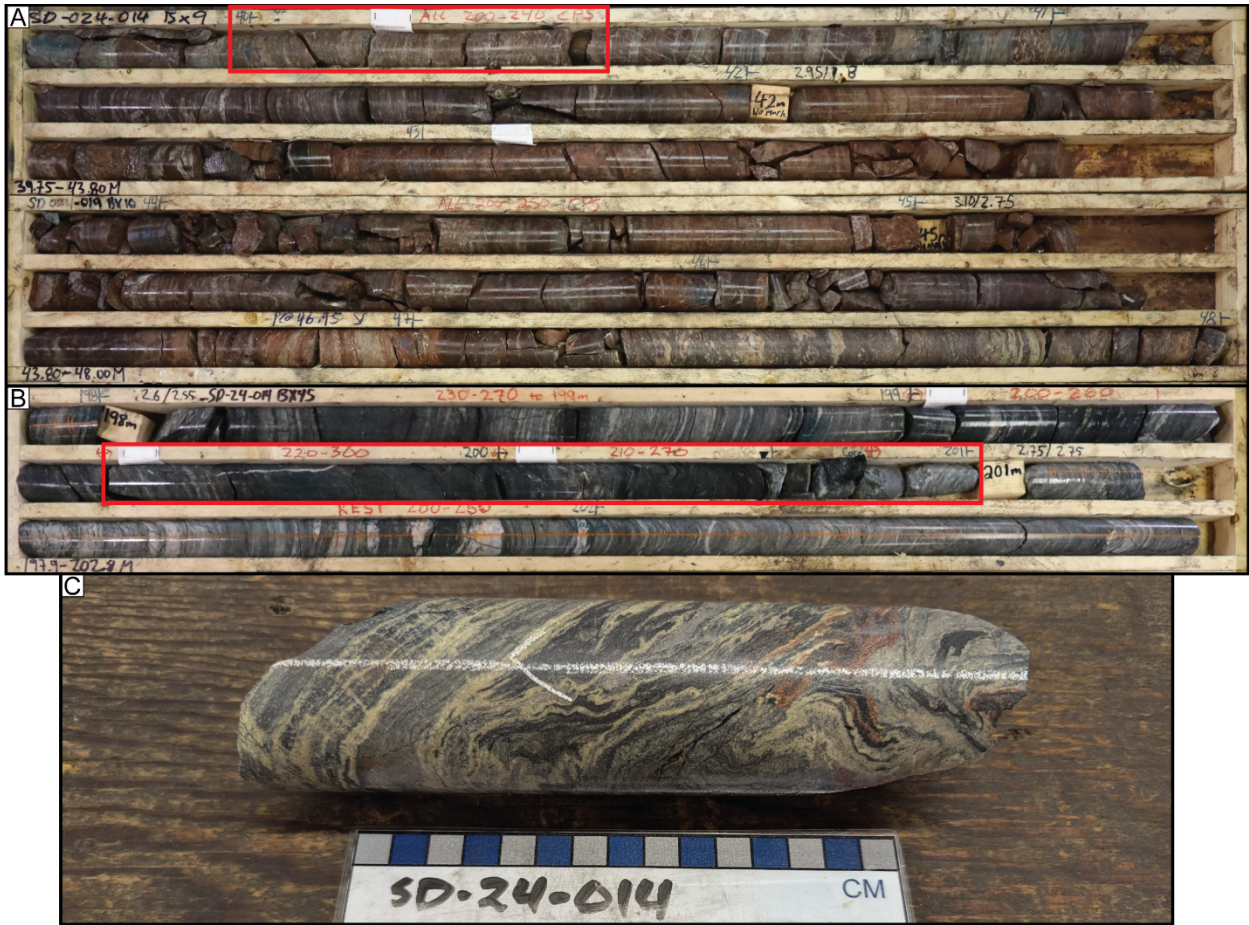
Figure 3. Drill core photos from hole SD-24-014 highlighting intervals of anomalous radioactivity, alteration and structure. A) Faulted and strongly hematized and clay-altered hangingwall rocks hosting radioactivity up to 369 cps at 40.0 m. B) Strongly graphitic footwall conductor hosting radioactivity up to 327 cps. C) Deformed pelitic rock exhibiting sericite-hematite alteration; Up to 250 cps, 122.7 m.
