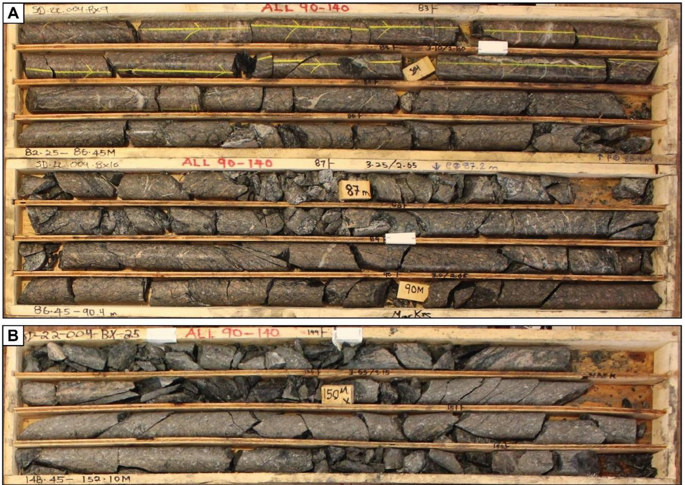
Figure 24. A) Brittle fault zone overprinting moderately clay-chlorite altered orthogneiss from 84.0 to 88.5 m in SD-22-004; up to 140 cps. B) Semi-brittle fault intersected from 146.8 to 150.5 m in SD-22-004 overprinting moderately altered orthogneiss; up to 140 cps.
