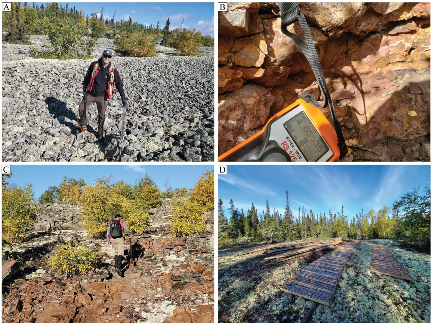
*Figure 43. A) Drill hole verification of Historic drill hole #7, B) The authors measuring radioactivity using RS-125 scintillometers on Stewart Island, C) The authors measuring radioactivity using RS-125 scintillometers at the JNW-1 deposit on Johnston Island, D) The Core Yard at the Sun Dog Project on Stewart Island*
