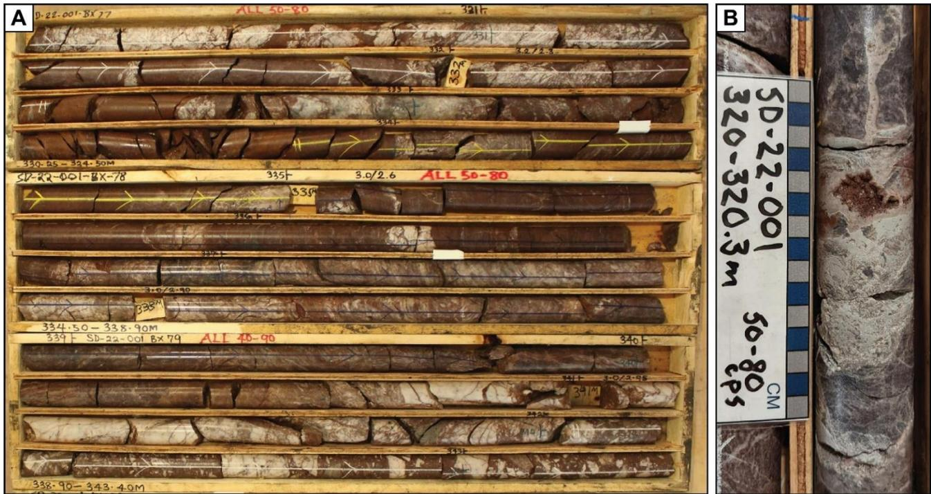
Figure 22. A) Metre-scale hydrothermal quartz-hematite breccias intersected in SD-22-001 basement rocks indicating repeated deformation and strong fluid flow in the Haven area. B) Hydraulic breccia containing white clay, dravite, and hematized drusy quartz in SD-22-001; 50-80 cps.
